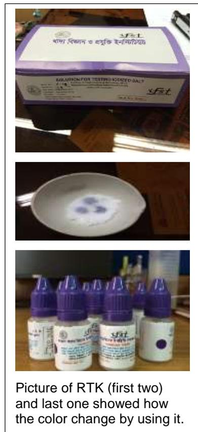
Picture of RTK (first two) and last one showed how the color change by using it.
